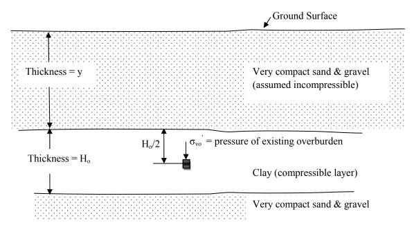
For upper sand and bottom sand stratum, y = 3.66 m,  $\gamma$  = 21.2 kN/m3
